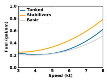
configurations on several vessels suggest that operating "tanked" typically increases fuel consumption about 20% and deploying stabilizers increases fuel consumption by about 40% when operating near cruising speeds.
