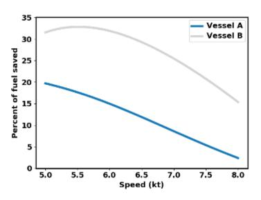
The Figure to the left shows how much fuel consumption can be reduced by cleaning the hull. The plot shows data from two sea trials performed before and after a hull cleaning. The data show a broad range in fuel consumption improvement depending on the vessel, but it appears that fuel consumption is typically reduced by around 15% at cruising speeds.
