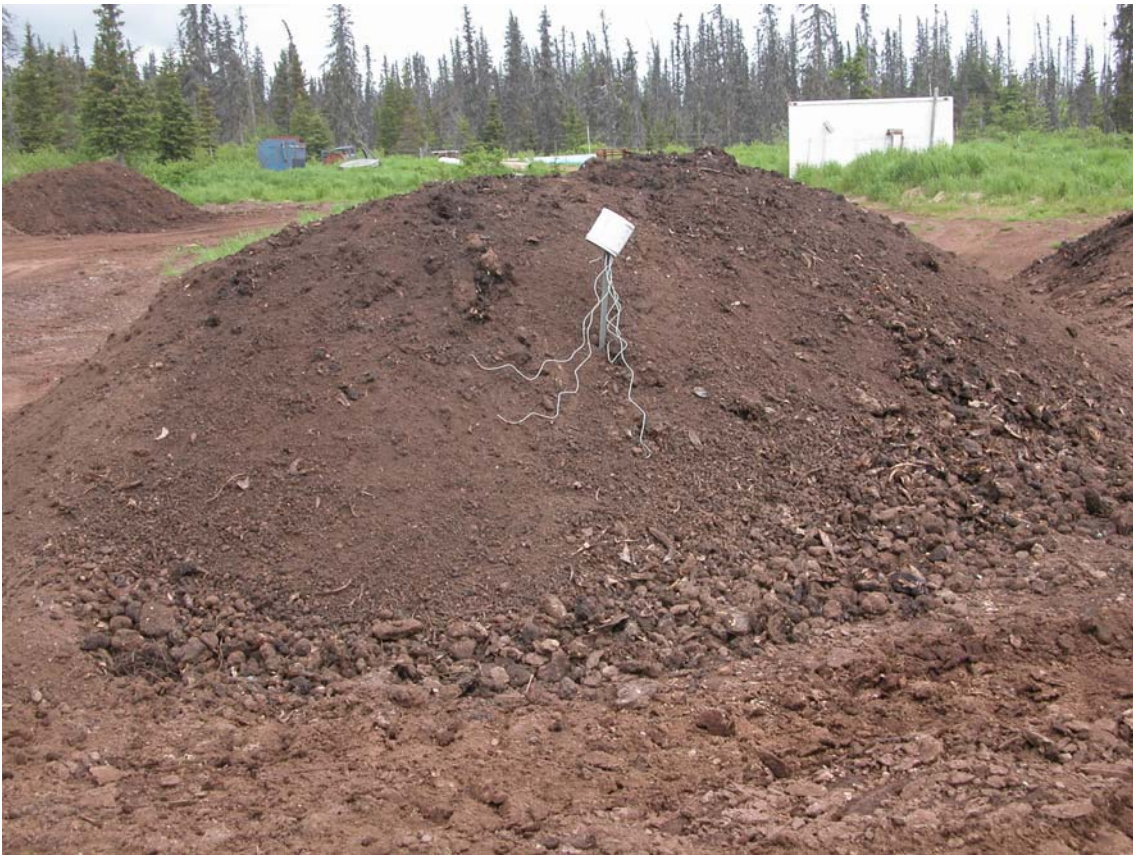
Plate 1. Compost pile set up in early June in the compost site of Ocean and Earth. The wires were temperature sensors, and below the bucket was the HOBO data log.
