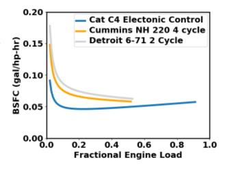
full power because the engines did not achieve their rating during the trial. The engines are fairly typical of two cycle, four cycle, and electronically governed engines surveyed by the Fishing Vessel Energy Efficiency Project (FVEEP). For all classes of engines, the fuel consumption is nearly constant between 50 and 100% of the continuous load rating, but increases rapidly as the load falls below 20%. That increase in BSFC illustrates the inefficiency of running an oversized engine.
