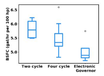
The data are manufacturer BSFC ratings at full load under a continuous use rating. The data show that electronically governed engines tend to be more efficient than mechanically governed engines, and that turbo charged engines tend to be more efficient at full load than naturally aspirated engines. However, there is overlap between each group of engines.
