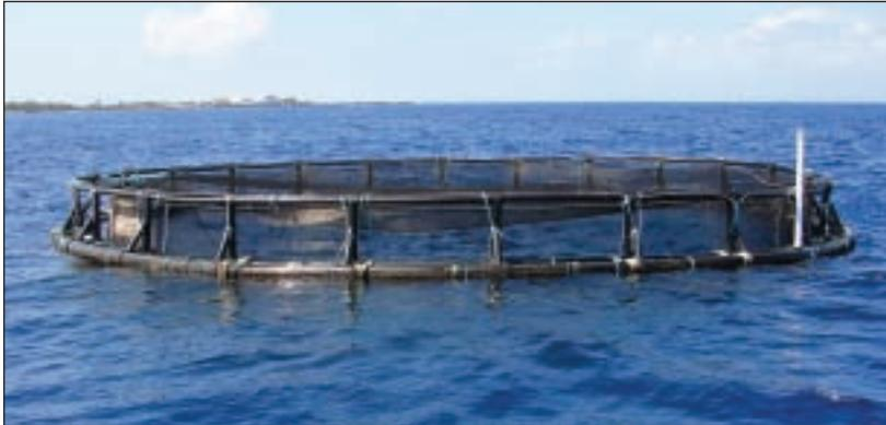
Net pens are typical of the equipment used to culture marine finfish in many parts of the world.
