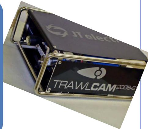
The new JT electric TRAWLCAM2008 is an autonomous deep water video recording system that has been specifically designed to provide a compact and robust unit for capturing underwater video data. The TrawlCam 2008 is design for and in conjunction with fishing trawler owners operating in the harsh environment in the North Atlantic Ocean near Faroe Islands and Iceland, and the Arctic Sea near Greenland.
